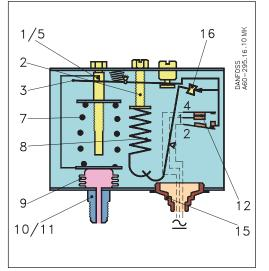
The switch in the KP has a snap-action function and the bellows moves only when the cut-in or cut-out value is reached.
