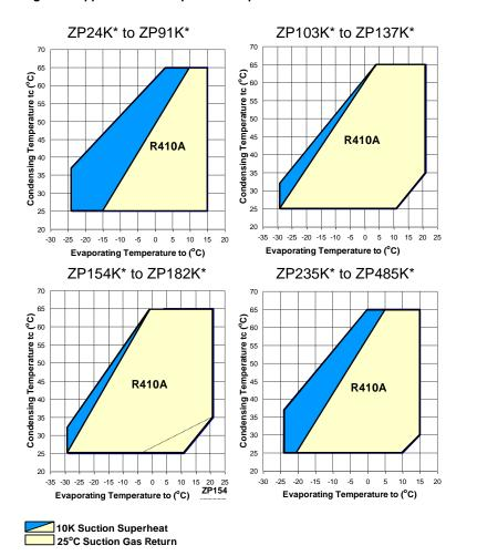
Figure 2: Application envelopes for compressors ZP24K\* to ZP485K\* with R410A
