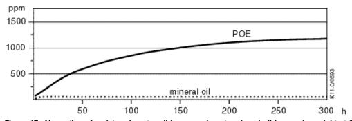
Figure 17: Absorption of moisture in ester oil in comparison to mineral oil in ppm by weight at 25°C and 50% relative humidity (h=hours)
