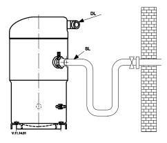
Figure 8: Suction tube design
