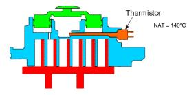
Figure 15: Internal discharge temperature sensor position
