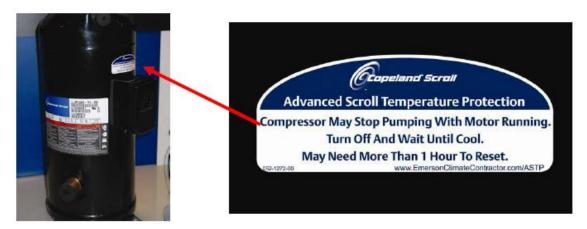
Figure 14: Advanced Scroll Temperature Protection (ASTP)
